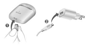
The internal battery starts charging. When hearing instruments are inserted, they start charging as well. The charging status of the charger is shown permanently.
